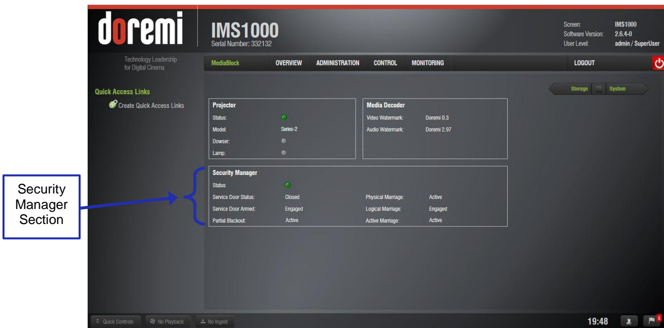
Figure 41: Security Manager Section
